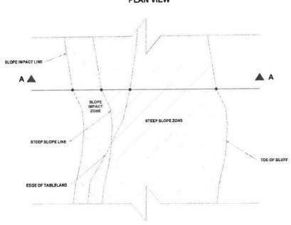
DETERMINING SLOPE IMPACT AREA FOR BLUFF WITH SIMPLE SLOPE PLAN VIEW
